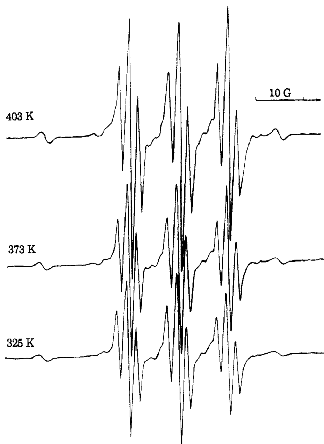
Figure 3. ESR spectra of the n\text{-C}_{24}\text{H}_{50} /BP/BNB sample irradiated at room temperature and recorded at different temperatures in the following order: (A) 403 K; (B) 373 K; (C) 325 K.
